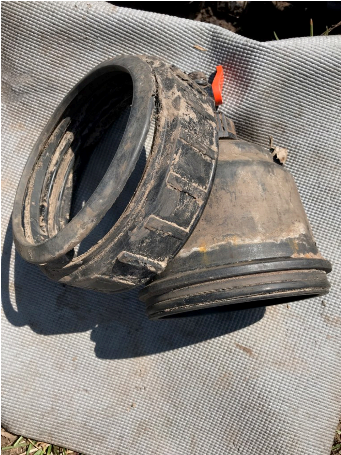
Cracked collar from filter enclosure.
